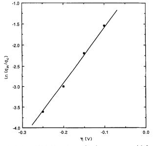
Fig. 8. Logarithmic dependence of  $q_{in}/q_c$  on overpotential for Inconel 718 at a charging time of 20 s.
