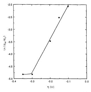
Fig. 9. Logarithmic dependence of  $q_{\rm in}/q_{\rm c}$  on overpotential for Hastelloy C-276 at a charging time of 20 s.
