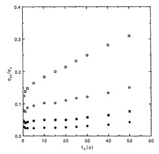
Fig. 4. Dependence of  $q_{\rm in}/q_{\rm c}$  on charging time for Inconel 718 at various overpotentials: (D) -0.10, (O) -0.15, (**B**) -0.20, (**O**) -0.25 V.
