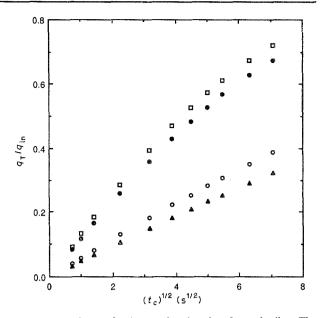
Fig. 3. Dependence of  $q_T/q_{in}$  on charging time for each alloy. The apparent rate constants are given in parentheses for the particular alloy: ( $\Box$ ) Inconel 718 (0.031); ( $\odot$ ) Incolog 925 (0.006); ( $\blacktriangle$ ) Inconel 625 (0.004); ( $\bullet$ ) Hastelloy C-276 (0.025).
