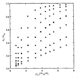
Fig. 1. Dependence of  $q_{\rm T}/q_{\rm in}$  on charging time for different values of  $k_a$ : ( $\Box$ ) 0.005, ( $\bullet$ ) 0.010, ( $\triangle$ ) 0.025, ( $\blacksquare$ ) 0.050, ( $\circ$ ) 0.100, ( $\diamond$ ) 0.200, ( $\triangle$ ) 0.500 s<sup>-1</sup>.
